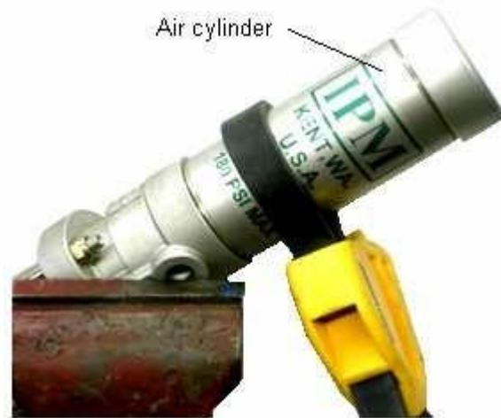
Remove the air cylinder either by hand or by using a strap wrench.
