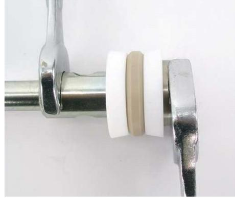
**Internal foot valve disassembled.** Once disassembled, clean and inspect each part, replace any parts if damaged prior to reassembling. Use threadlocker when re-installing.
