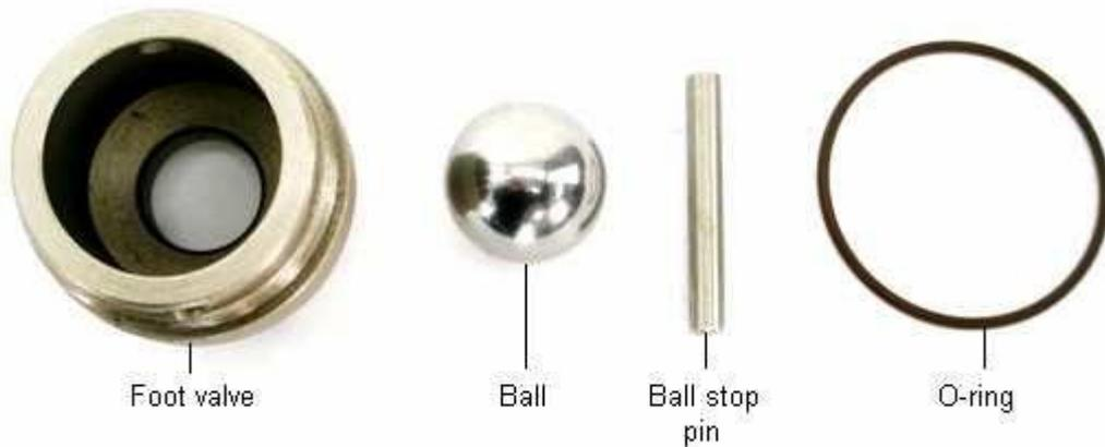
**Lower foot valve parts.** On the **stubby** version of the IP02 pump there are 3/4" female pipe threads under the foot valve- on the **drum length** there are not. Should you need to extend into your container farther it is recommended to install a cylinder extension tube to keep the foot valve at the lowest possible point.
