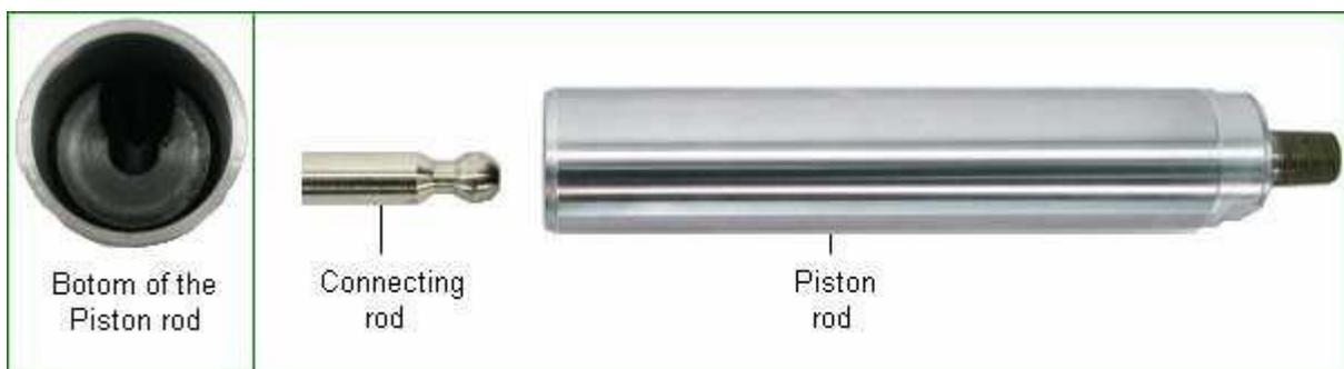
The pump assembly can be removed from the air motor by disengaging the Piston Rod.
