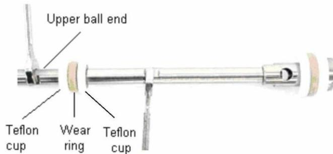
3. Use two wrenches and dismantle the upper pump section. Note the orientation of the Teflon cups. One faces up, followed by a wear ring in the center and the second cup faces down followed by a lower support washer. Use threadlocker when re-installing.
