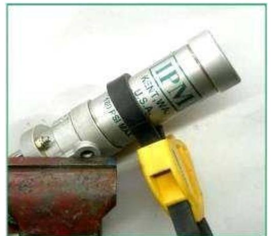
15. From fluid section, unscrew displacement rod from the piston shaft. Examine for debris build-up or damage. Re-assemble the muffler with the point of the cone facing up inside the piston shaft. Screw the displacement rod into the piston shaft.
