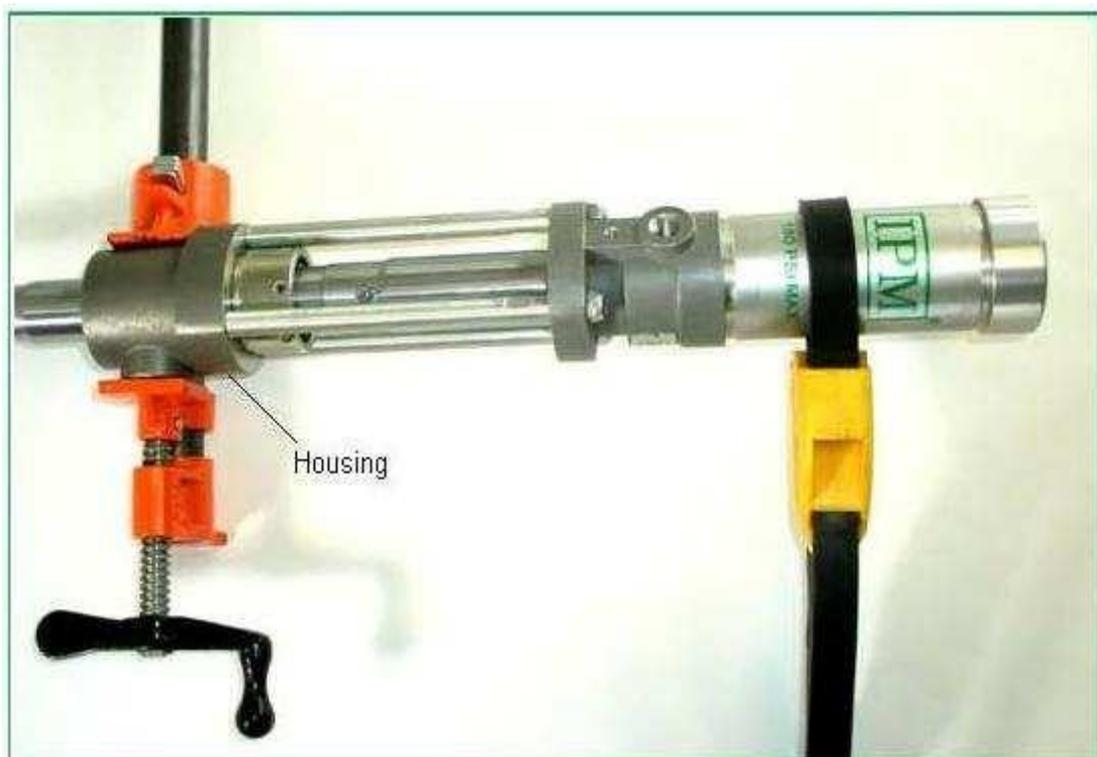
3. Remove the foot valve, while holding the air cylinder with a strap wrench as shown.
