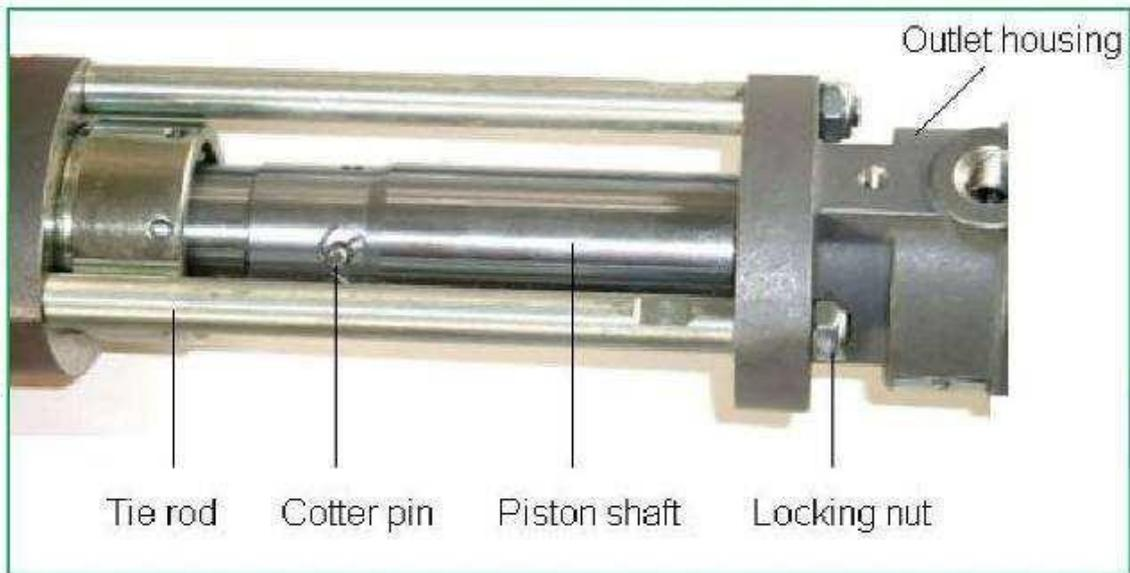
12. From the air motor section, remove the cotter pin then remove the flat head pin. Unscrew the displacement rod from the piston shaft, as shown in diagram above.
