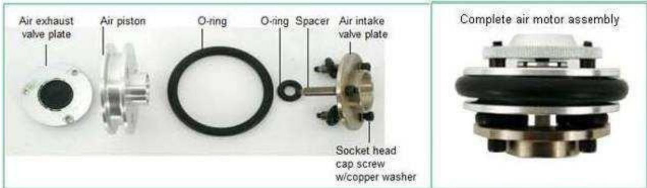
2. Assemble the complete air motor assembly again using threadlocker with washer onto the piston shaft. Hand-tighten only.
