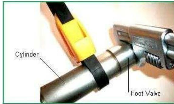
4. Use snap ring pliers to remove snap ring and E-clip. Remove check ball and examine foot valve for debris and/or damage. Replace as necessary. Replace Teflon O-ring and re-assembly foot valve with ball, snap ring and E-clip.
