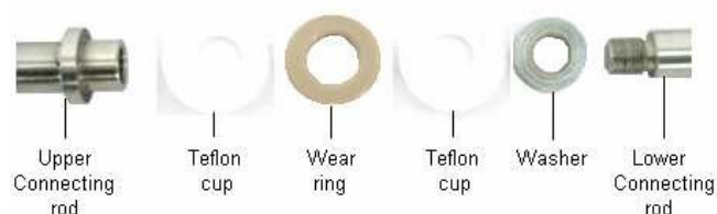
Breakdown of upper portion of the lower connecting rod assembly.
